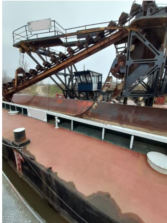
Figure 6.2. Bucket elevator (unloader) for gravel
