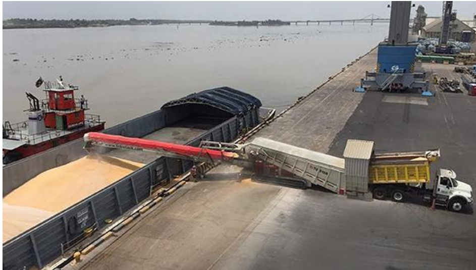
Figure 6.4. Hopper loader with belt conveyor
