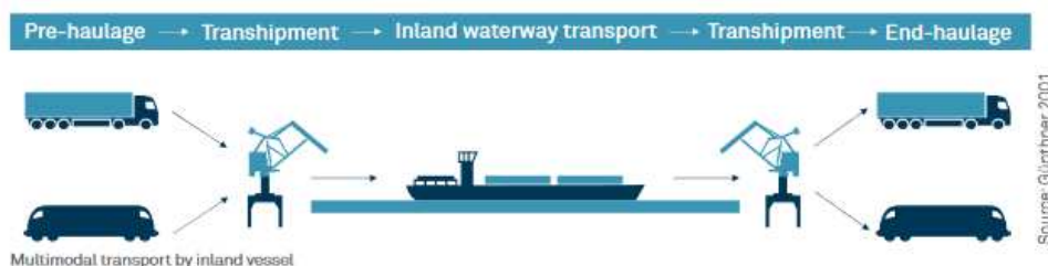
Figure 2: Steps in the multimodal transport by inland vessel (Source: viadonau)
