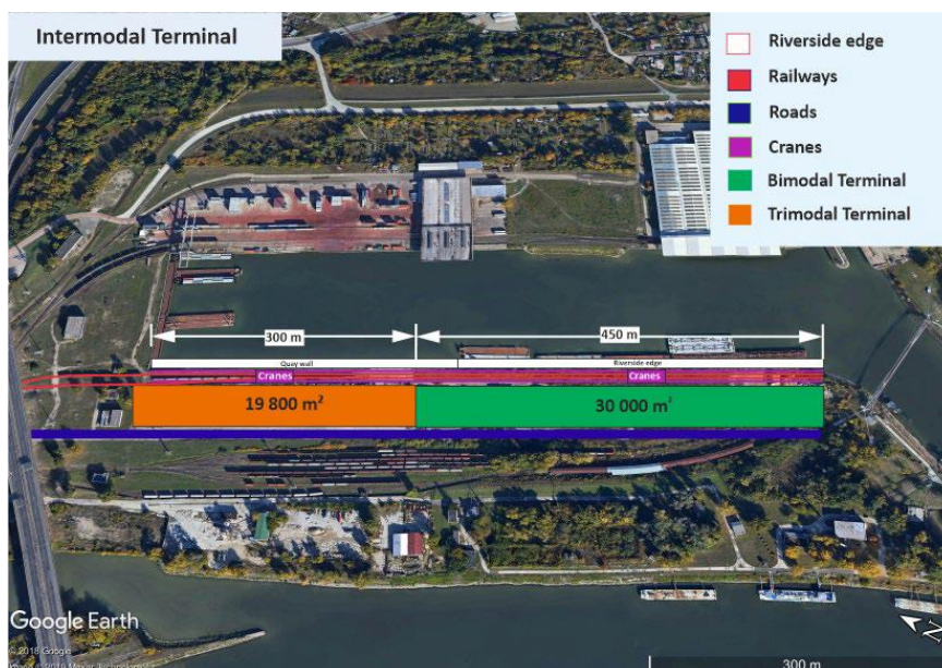
Figure 12: Layout of intermodal terminal Bratislava - ŽSR project 2
