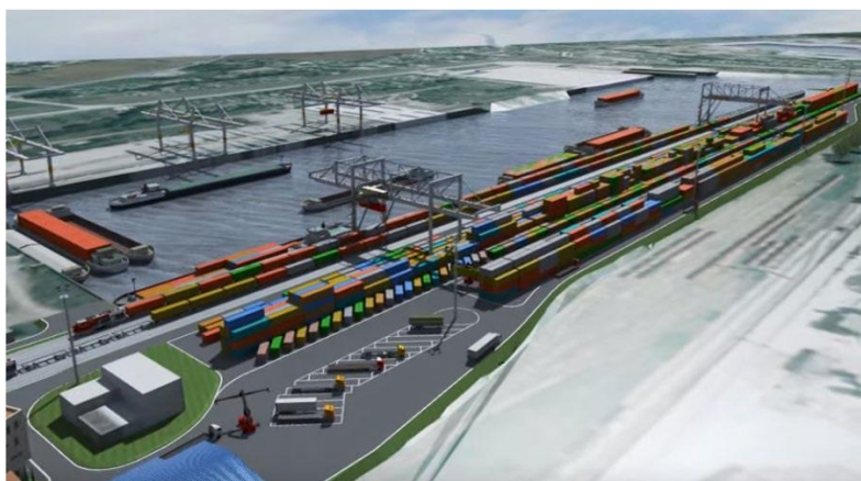
Figure 11: Layout of intermodal terminal Bratislava - ŽSR project 1
